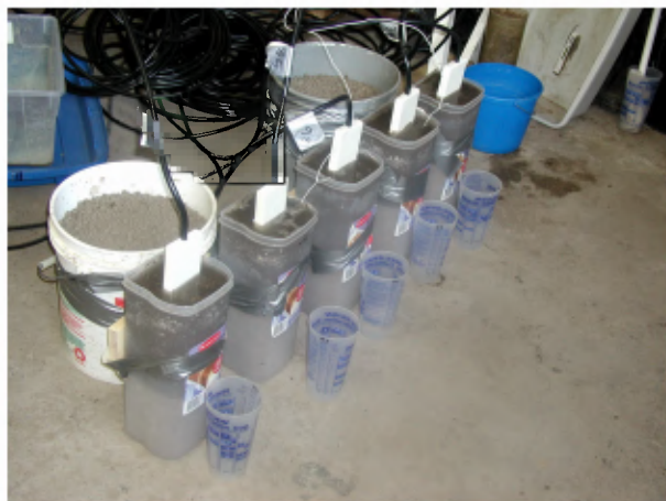
Figure 2. Performing soil TDR experiments in the laboratory.
