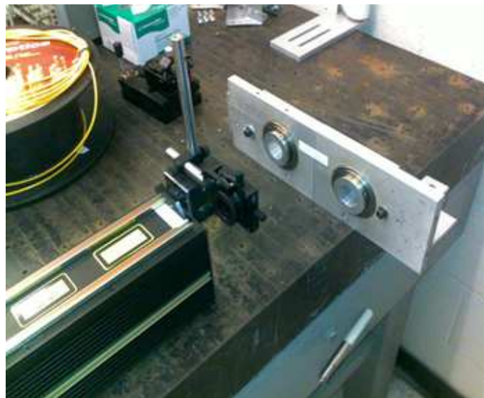
Figure 2.2: Schematic of the \pi FBG fabrication setup (left), reflection spectrum of the original regular FBG and during the CO 2 laser heating process (right), and image of the physical setup (Bottom).
