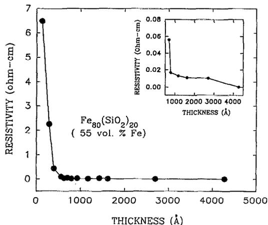
FIG. 3. Resistivity vs thickness for the  $\text{Fe}_{80}(\text{SiO}_2)_{20}$  films.
