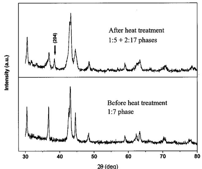
FIG. 1. X-ray diffraction pattern (a) before and (b) after annealing. The arrow shows a characteristic 2:17 peak.
