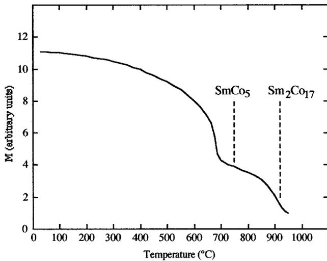
FIG. 2. Thermomagnetic analysis of  $\text{SmCo}_{6.1}\text{Cu}_{0.6}\text{Ti}_{0.3}$  magnet. The dashed lines show the Curie temperatures of the pure  $\text{Sm}_2\text{Co}_{17}$  and  $\text{SmCo}_5$  phases.
