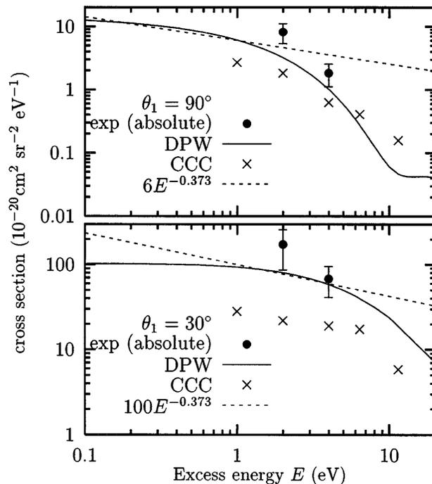
FIG. 2. Equal energy sharing  $e$ -H triply differential cross sections at  $\theta_1 = 90^\circ$  and  $30^\circ$  in the Wannier ( $\theta_{12} = \pi$ ) geometry as a function of excess (total) energy.
