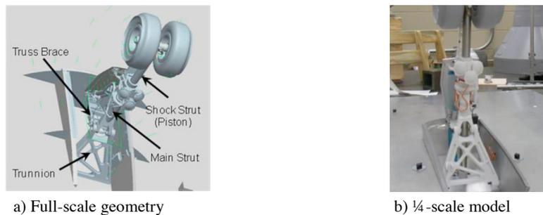
Fig. 3 Difference between full-scale and model-scale nose gear geometries at junction of main strut, trunnion, and truss brace.
