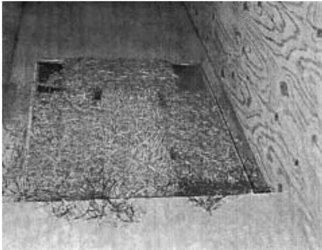
Figure 4—Measuring thermal resistance of Bermudagrass sods.
