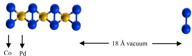
Fig. 1. Atomic structure of the considered Pd–Co thin film. Both the top and the bottom of the film are Co-terminated, which is important for the physical understanding of the ME effect.
