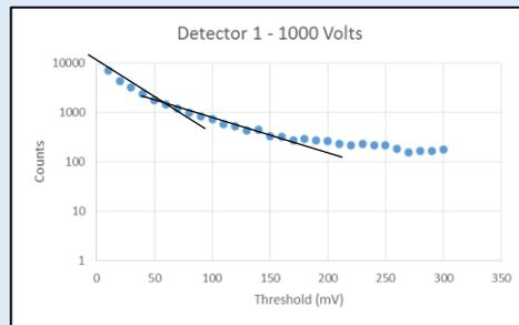
Figure 3 – Threshold Scan at 1000 Volts
