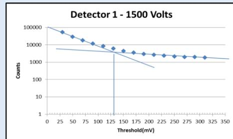
Figure 2 – Threshold Scan at 1500 Volts
