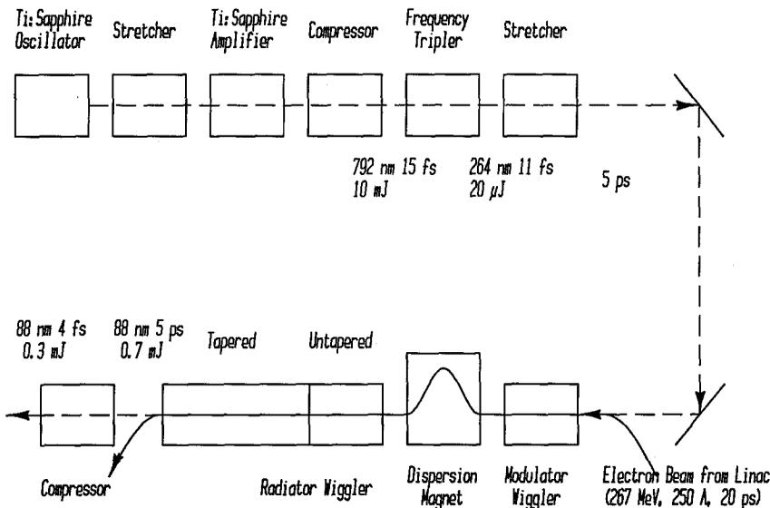
FIG. 1. A schematic diagram showing the experimental arrangement.
