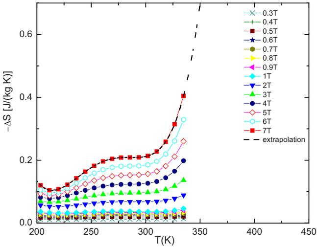
FIG. 7. (Color online) Temperature dependence of the mass specific entropy change  $\Delta S$  calculated from Eq. (15), using the experimental isotherms in the temperature interval  $120 \leq T \leq 330$  K measured in steps of  $\Delta T = 10$  K to numerically calculate  $\frac{\partial m}{\partial T}$  vs  $\mu_0 H$  for  $0 \leq \mu_0 H \leq 7$  T. The dotted line shows an extrapolation of  $-\Delta S$  vs  $T$  toward higher temperature going beyond our experimental data.
