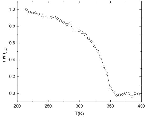
FIG. 2. Normalized magnetic moment  $m/m_{\max}$  vs  $T$  of noninteracting ultrathin Co films after zero-field cooling and subsequent field heating in  $\mu_0 H = 5$  mT. The Curie temperature of bulk Co has been reduced by more than 1000 K due to a geometrical confinement of the correlation length perpendicular to the film plane.
