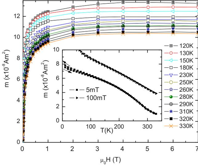
FIG. 6. (Color online) Isotherms  $m$  vs  $\mu_0 H$  for  $0 \leq \mu_0 H \leq 7$  T. The inset shows field heating and cooling  $m$  vs  $T$  data at 5 mT (squares) and 100 mT (triangles). All curves are initialized by zero-field cooling, and the arrows indicate the direction of the temperature change.
