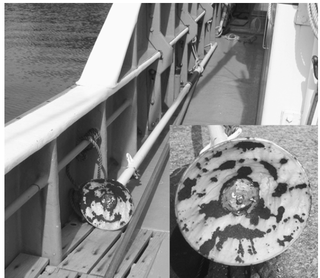
Fig. 1. The trumpet used to produce sound in the drive fisheries operating out of Taiji, Japan, consists of a metal pole, about 2.9-4.5m long, with a concave metal disk, about 22-26cm in diameter, attached to the bottom. One trumpet is used on each side of the boat. The fishermen place the disk end of the trumpet in the water and strike the pole with a hammer approximately every 2s, creating an acoustic barrier that helps the collection vessels herd schools of small cetaceans into the harbour. The insert shows a close-up of the concave disk that produces the sound.
