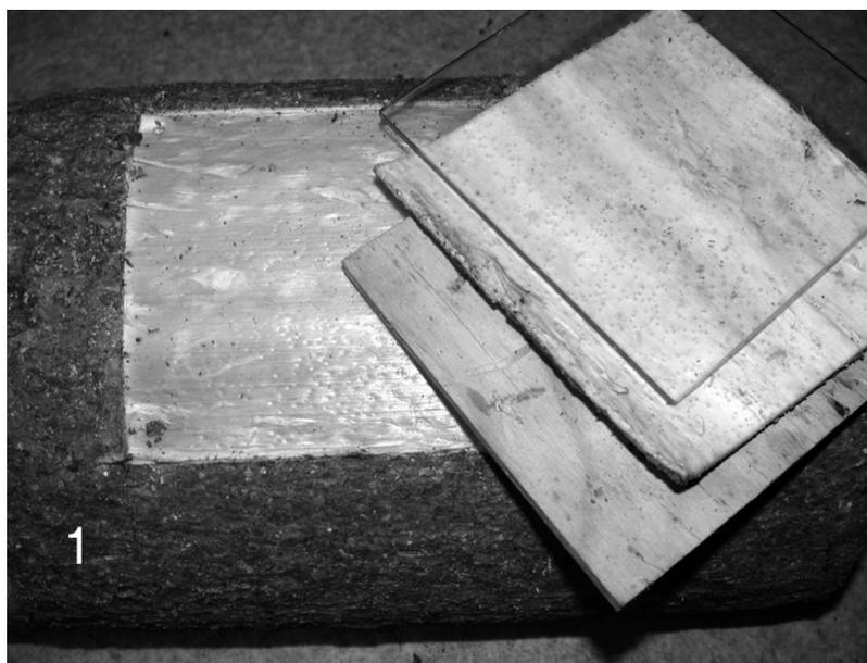
Fig. 1. Preparation of a phloem plate for rearing and observation of *D. murrayanae* in the laboratory. A piece of bark, removed from a freshly felled lodgepole pine, is shown sandwiched between plywood backing and plate glass. After inserting a stage of the beetle, the sandwich will be held together with masking tape.
