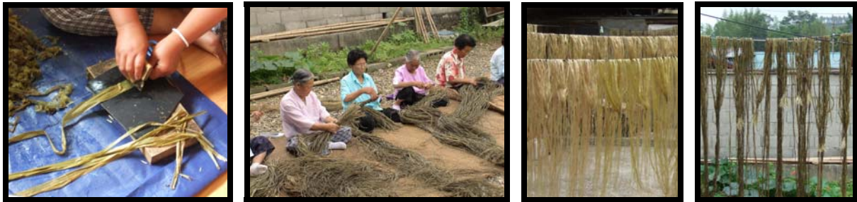
Figure 9. (left) Scraping epidermis off the hemp fiber layers in Andong. (left-center) Softening the thicker ends of the fiber layers in Boseong. Photographs by the author.
