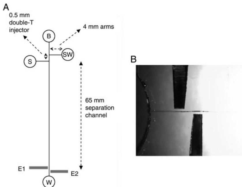
**Figure 1.** Schematic diagram of the microchip (A) and detailed view of electrode alignment (B). Channel width: 50  $\mu\text{m}$ , channel depth: 50  $\mu\text{m}$ , double T arms: 4 mm long, solution reservoirs: 5 mm diameter. S, sample reservoir; SW, sample waste reservoir; B, BGE reservoir; W, waste reservoir; E1, input electrode and E2, output electrode.
