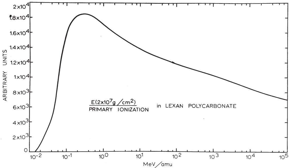
**Figure 5.** The ratio of two criteria for track formation in dielectrics: energy deposition at  $\times 10^{-7} \text{ g/cm}^2$  <sup>(5)</sup> / total primary ionization(s) in Lexan polycarbonate. If these criteria are calibrated by bombardment with machine accelerated ions at 1-10 MeV/amu, the changing ratio of the two criteria implies that the energy deposition criterion will yield a higher identification for relativistic ion tracks than will the primary ionization criterion.
