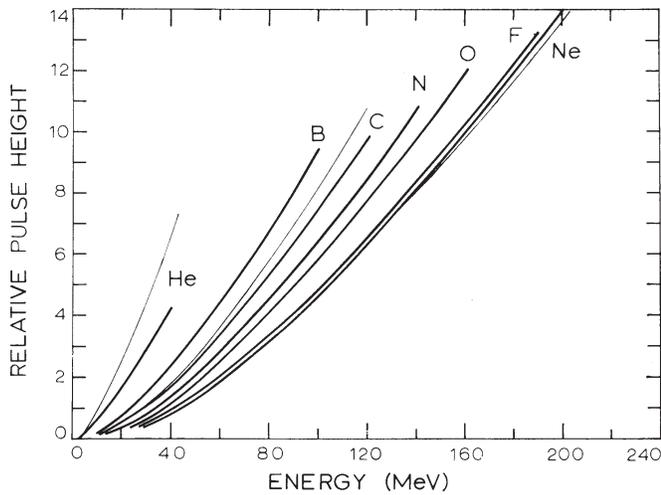
**Figure 3.** Experimental values of relative pulse height in NaI(Tl) from a spectrum of incident ions plotted against ion energy as light lines, while normalized theoretical results are plotted as heavy lines. In some cases the light lines are obscured by the heavy lines. (Katz and Kobetich, 1968-2).
