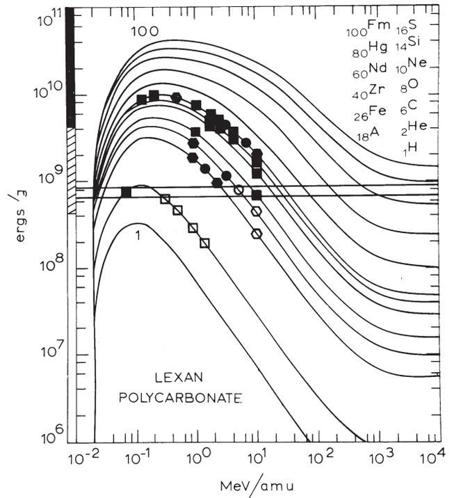
**Figure 4.** Dosage of ionization energy in Lexan polycarbonate at  $2 \times 10^{-7} \text{ g/cm}^2$  ( $17 \text{ \AA}$ ) from the ion's path for a spectrum of ions and ion energies. Superimposed experimental points are solid if etchable tracks are formed, and are hollow if not.<sup>(5)</sup>
