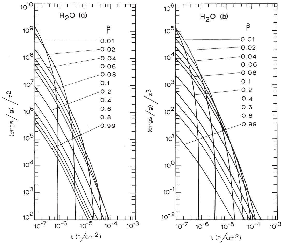
**Figure 1.** Spatial distribution of ionization energy,  $E(t)/z^2$ , in water as a function of the distance  $t$  from the ion's path, calculated from the  $\delta$ -ray distribution formula, and the assumption of normal ejection. Applicable to organic materials, where interest centers relatively close to the ion's path.<sup>(4)</sup> To find the energy deposition at distance  $t$  the contribution from (a) must be added to that from (b).
