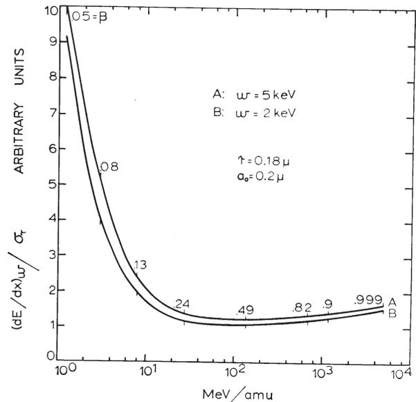
**Figure 7.** The ratio of two criteria for grain counts:  $(dE/dx)_{\text{restricted}}$  (in AgBr)<sup>(1)</sup>/ $\sigma\tau$ <sup>(6)</sup>
