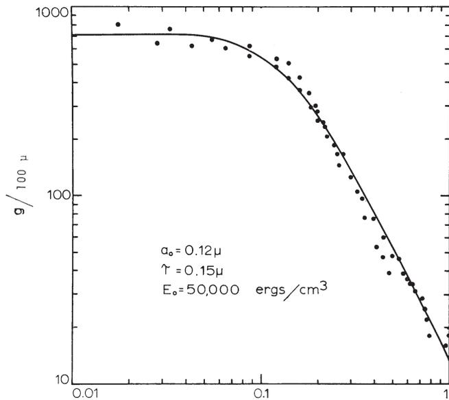
**Figure 6.** Grain count in K-5 emulsion for singly charged particles<sup>(9)</sup> as a function of  $\beta$ , plotted as points, while theoretical calculations are plotted as a line.<sup>(6)</sup>
