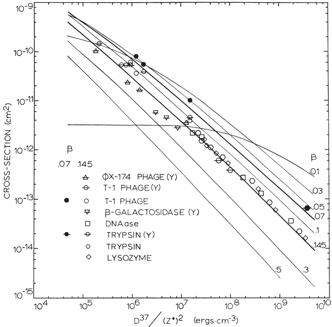
**Figure 2.** Cross section for the inactivation of dry enzymes and viruses, in relation to the critical dose ( $E_0 = D^{37}$ ) divided by the square of the effective charge of the bombarding ion. Plotted points crossed with a horizontal bar were obtained at the Yale HILAC (Y), while other points were obtained at the Berkeley HILAC. Lines arise from the theory.<sup>(2)</sup>
