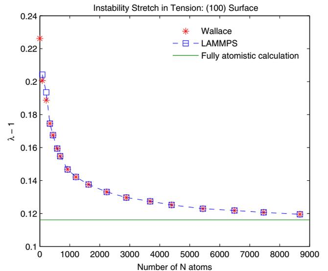
**Fig. 7.** Instability stretch comparison for the  $\langle 100 \rangle$  surface of an FCC crystal under uniaxial stretch along a  $\langle 100 \rangle$  direction as calculated using direct atomistic simulation (LAMMPS), the nonlocal Wallace criterion, and a thin film that is periodic in the plane with a free  $\langle 100 \rangle$  surface (fully atomistic calculation).
