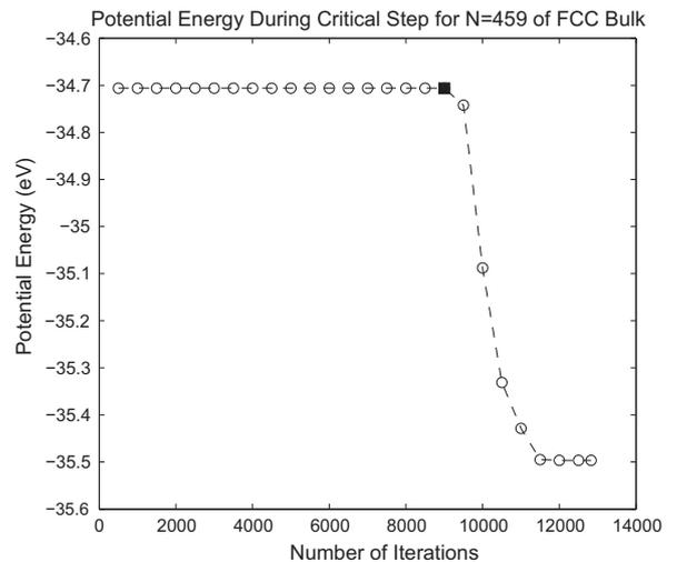
Fig. 4. Potential energy for the  $N = 459$  atoms versus the number of iterations during the energy minimization process for the critical (instability) step for tension of the bulk FCC crystal, where the exact point of instability is marked by the square around iteration 9000.
