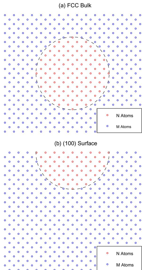
Fig. 1. (a) Spherical region  $\Omega$  in a bulk FCC crystal that contains the  $N$  atoms that participate in the failure process surrounded by  $M$  atoms; (b) hemispherical region used to analyze (100) surface instabilities that contains the  $N$  atoms that participate in the failure process surrounded by  $M$  atoms.
