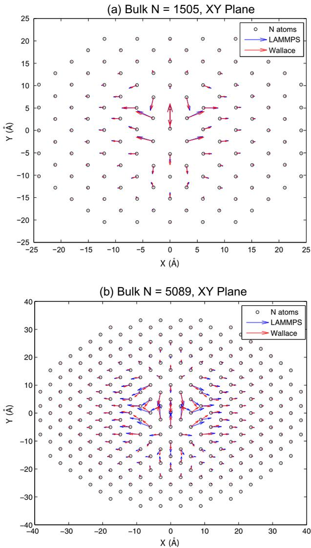
**Fig. 6.** Comparison of Wallace eigenvectors and LAMMPS displacement vectors on the  $xy$  plane for uniaxial stretching along a  $\langle 100 \rangle$  direction for a bulk FCC crystal using (a)  $N = 1505$  atoms, and (b)  $N = 5089$  atoms.
