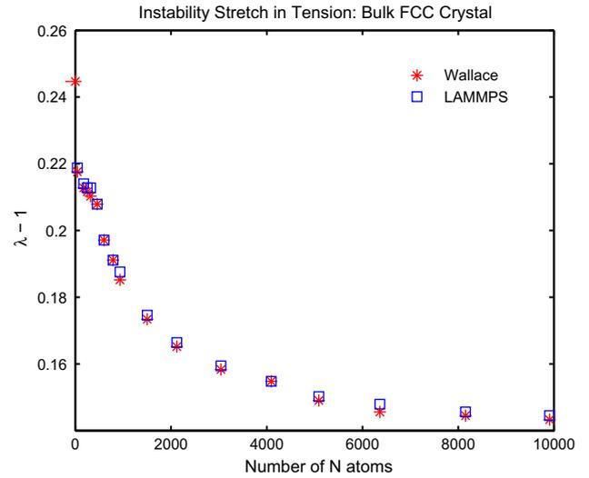
Fig. 3. Instability stretch comparison for a bulk FCC crystal under uniaxial stretch along a  $\langle 100 \rangle$  direction as calculated using direct atomistic simulation (LAMMPS), and the nonlocal Wallace criterion.
