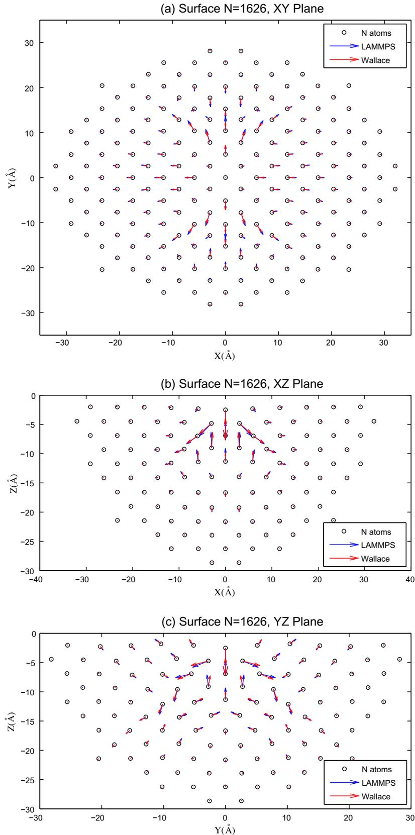
**Fig. 8.** Comparison of eigenvectors as calculated from Wallace formulation and displacement vector from fully atomistic simulation at onset of instability as shown for (a)  $xy$ , (b)  $xz$  and (c)  $yz$  planes for the (100) surface with  $N = 1626$ .
