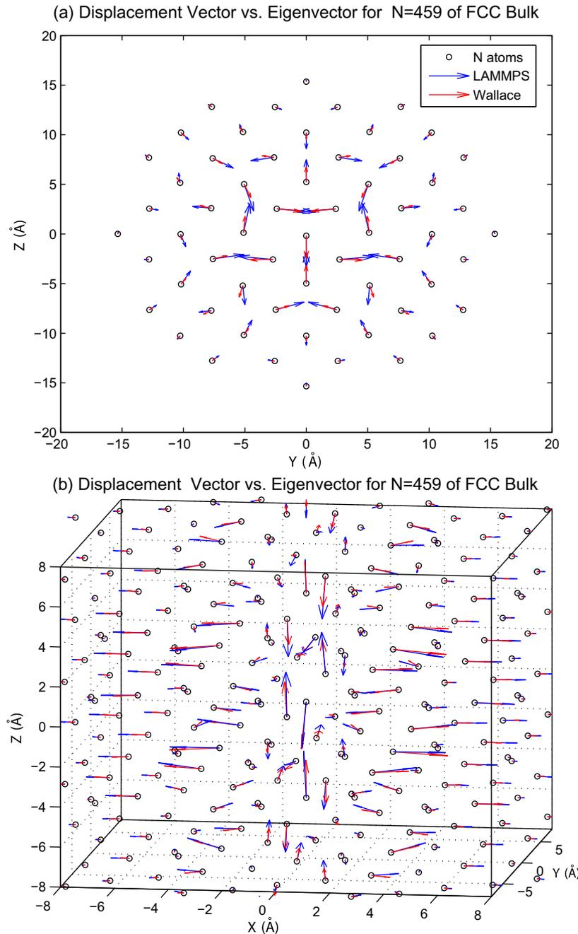
Fig. 5. Comparison of eigenvectors as calculated from Wallace formulation and displacement vector from fully atomistic simulation stretching a bulk FCC crystal along a  $\langle 100 \rangle$  direction at onset of instability depicted in Fig. (4) for  $N = 459$  as shown in both (a) 2D view of the  $yz$  plane at  $x = 0$ , and (b) fully 3D plot.
