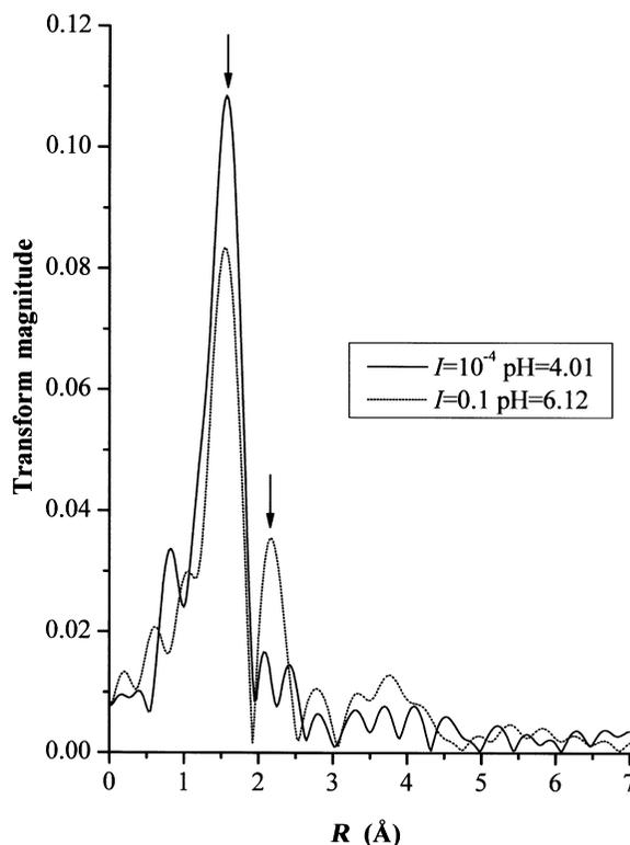
Figure 5. Fourier transform modulus for Cu sorbed on montmorillonite at pH = 6.12 and high ionic strength, and pH = 4.01 and low ionic strength ( $\Delta k = 3.4-11.8 \text{ \AA}^{-1}$ ). Samples are plotted on the same ordinate scale to illustrate the magnitude of second-shell backscattering contributions. The arrows indicate first- and second-shell backscattering features.
