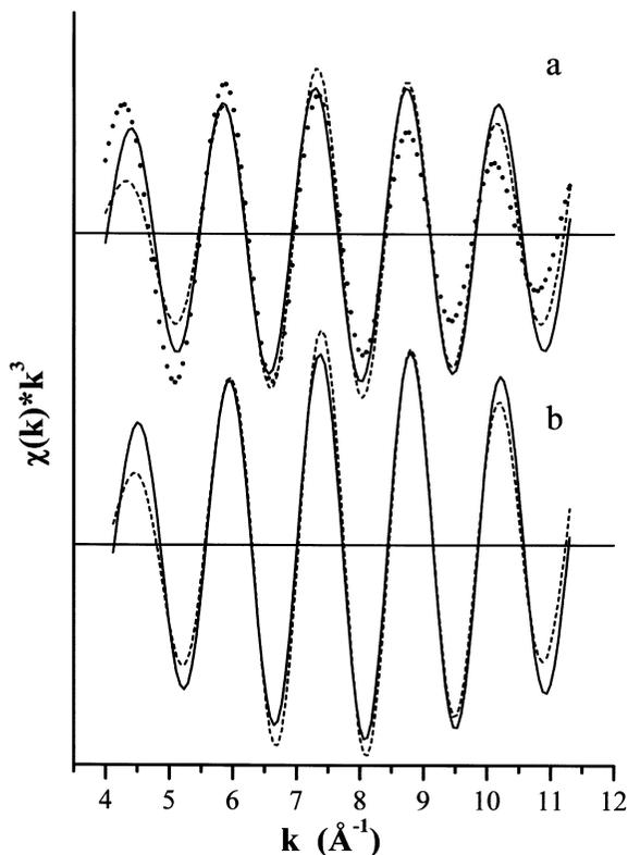
Figure 6. Backtransforms ( $\Delta R = 1.9\text{--}2.5 \text{ \AA}$ ) of (a) second shell in Fourier transform modulus of montmorillonite sample incubated at  $I = 0.1$  pH = 6.12, and (b) Cu acetate sample. The dashed lines are best fits using a single Cu backscatterer atom and the dotted line in panel a is best fit using a single Al backscatterer atom.
