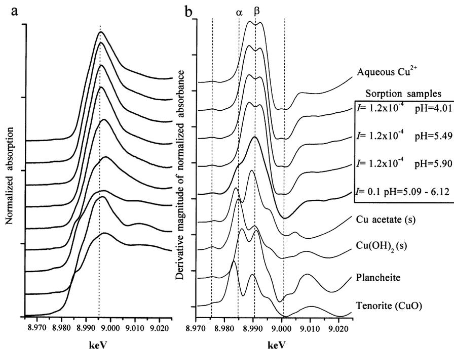
Figure 2. (a) XANES and (b) first derivative of XANES of Cu sorbed onto montmorillonite and selected reference materials. Vertical dashed lines are aligned with peaks of interest. *I* = 0.1 XANES is an average of three different samples (see text).
