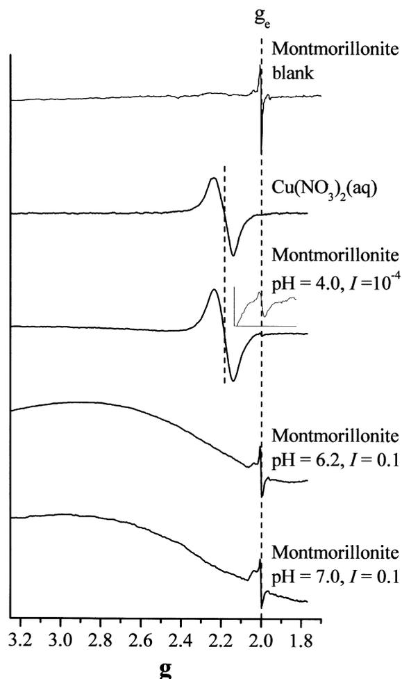
Figure 7. EPR spectra of Cu sorbed on montmorillonite as a function of pH and ionic strength.  $g_e$  is the free electron resonance at 2.003. A montmorillonite blank sample (no Cu) and aqueous  $\text{Cu}^{2+}$  EPR spectra are shown for reference. Inset on montmorillonite is zoomed in to show features since ordinate scales are different for each spectra.
