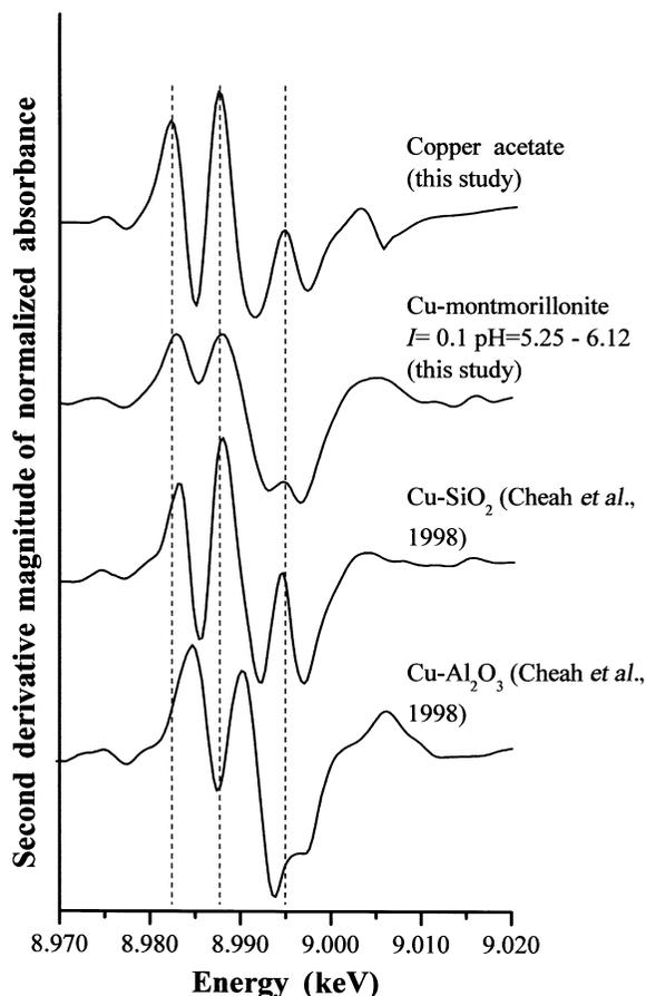
Figure 8. Comparison of second-derivative spectra from montmorillonite samples incubated at high *I* averaged (see text) with results from Cu sorbed on amorphous  $\text{SiO}_2$  and  $\text{Al}_2\text{O}_3$  as reported by Cheah *et al.* (1998). The Cu acetate spectrum was used to correlate the energy of the samples in the two studies.
