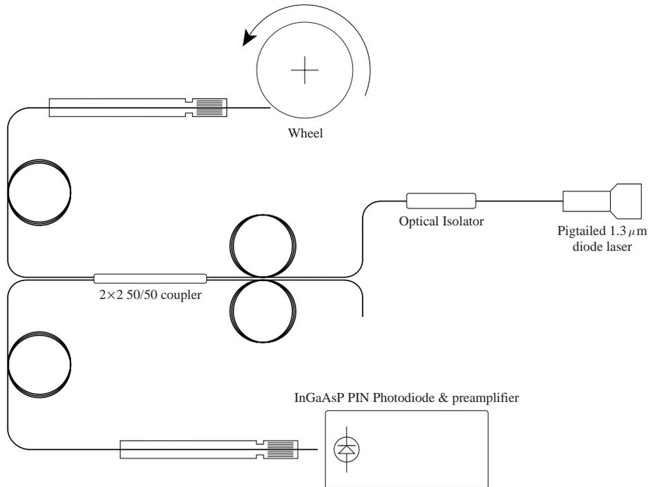
FIG. 1. Experimental setup for fiber-optic laser Doppler velocimeter.
