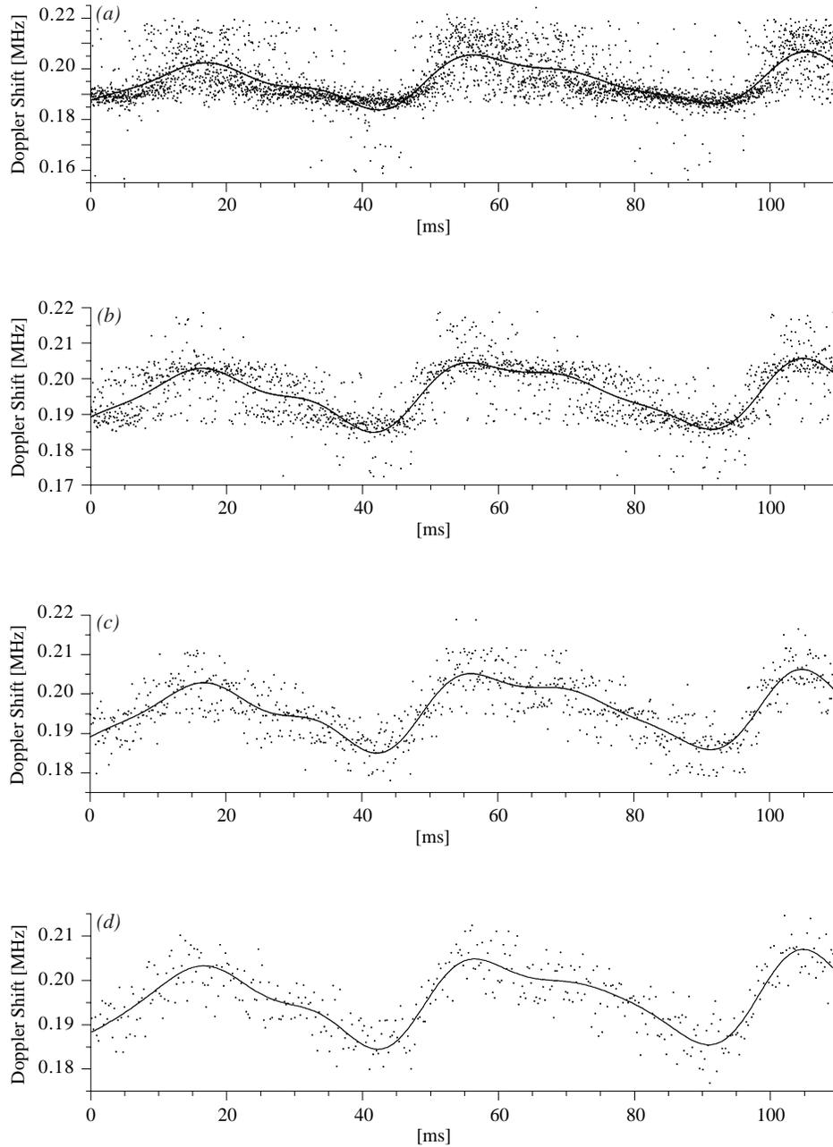
FIG. 5. Best fit (solid line) and raw time series (dots) using (a)  $32 \mu\text{s}$ , (b)  $64 \mu\text{s}$ , (c)  $128 \mu\text{s}$ , and (d)  $256 \mu\text{s}$  windows. The best fits correspond to the parameters shown in Table (I).
