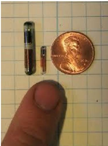
**Figure 2:** 12mm and 8mm PIT tag comparison
