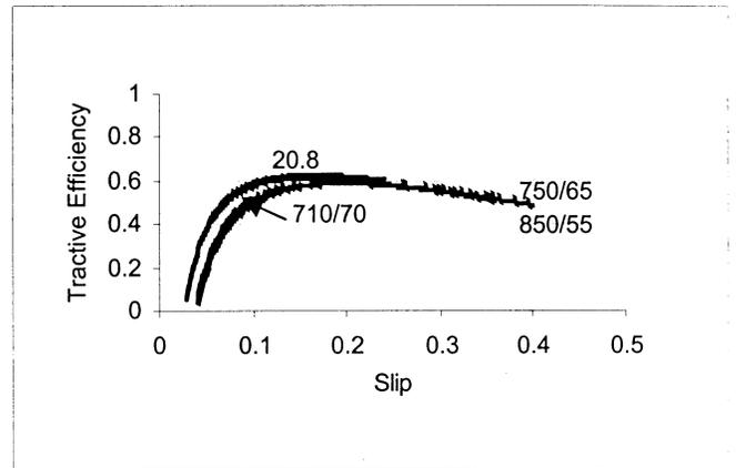
Figure 4. Tractive efficiency vs. slip for the designated tires on a tilled wheat stubble field.
