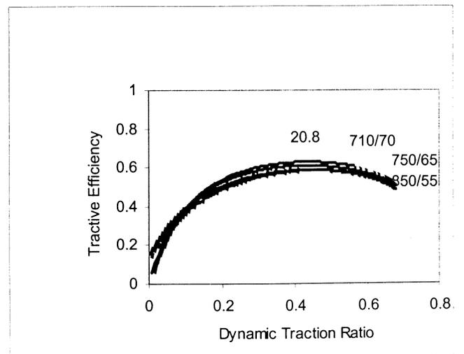
Figure 6. Tractive efficiency vs. dynamic traction ratio for the designated tires on a tilled wheat stubble field.
