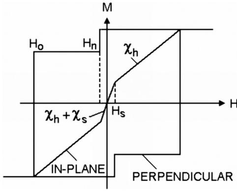
FIG. 4. Effect of exchange coupling on the hysteresis of hard-soft composites. Note that  $H_0/H_n \approx 1.5$ , depending on the geometry of the inclusion.  $\chi_h$  and  $\chi_s$  represent the slopes of the in-plane loop due to the hard and soft phase, respectively, and for macroscopic inclusions,  $H_s = H_n = 0$ .
