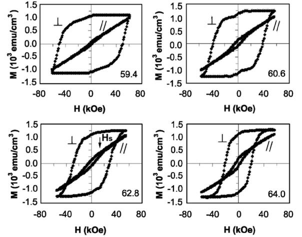
FIG. 3. Room temperature hysteresis loops of the Fe-Pt films with different Fe concentrations, as labelled. The in-plane and perpendicular loops are indicated by ( $\parallel$ ) and ( $\perp$ ), respectively. The field  $H_s$  (see text) is indicated in  $x = 62.8$  loop.
