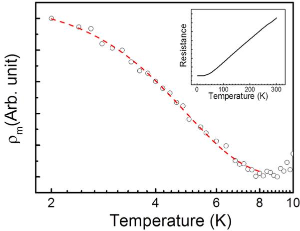
FIG. 1. Temperature dependence of resistivity of the film sample  $\rho_m = \rho - \rho_{\min}$  between 2 K and 11 K. The dashed line represents the NRG fitting. The inset shows resistivity as a function of temperature measured between 2 K and 300 K.
