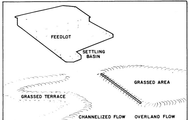
FIG. 1 Vegetative filter configurations for feedlot runoff treatment.
