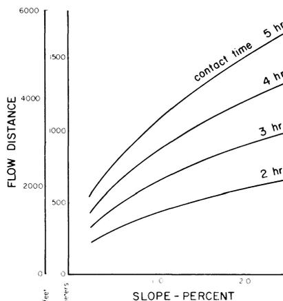
**FIG. 2 Approximate channelized-flow distance required for various slopes and contact times.**
