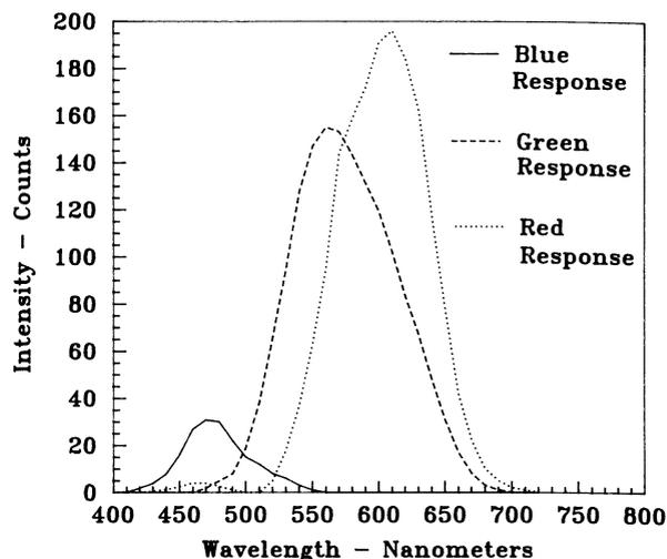
**Fig. 5—C.I.E. weighted spectral intensity versus wavelength for corn residue cover.**
