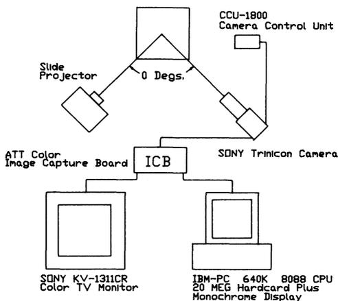
Fig. 1b—Layout for color (ICB) image processing system.
