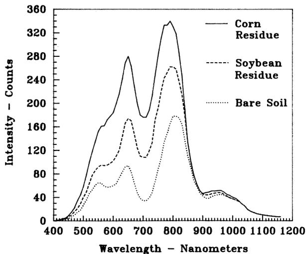
**Fig. 4—Spectral intensity versus wavelength for soil-residue components.**
