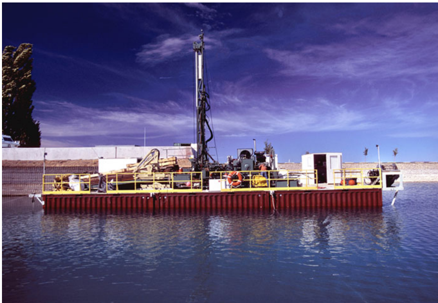
Fig. 1 The GLAD800 drill rig and platform ( RV Kerry Kelts ) at the Bear Lake Marina, Garden City, Utah
