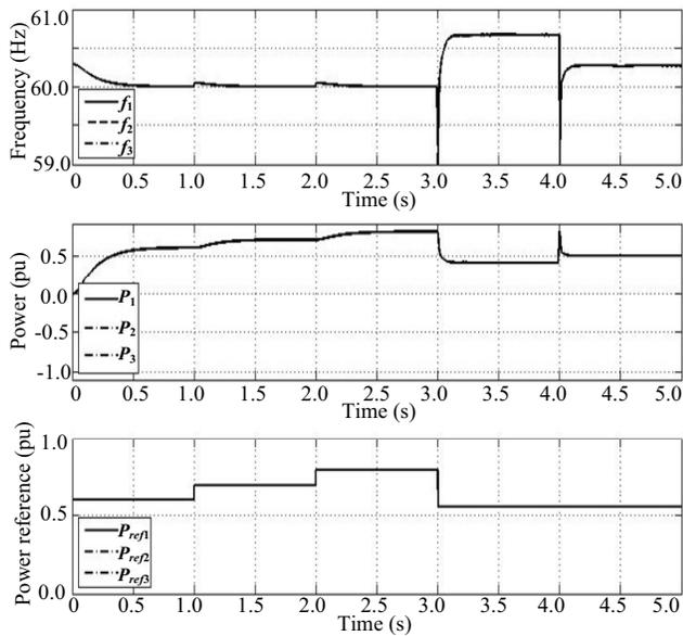
Fig. 6. Load changes from 1.2 pu to 1.5 pu but the reference power has no change at 3 s and 4 s
