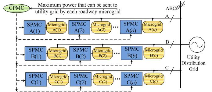
Fig. 2. The architecture of multiple single-phase roadway microgrids integrated into a three-phase distribution grid.
