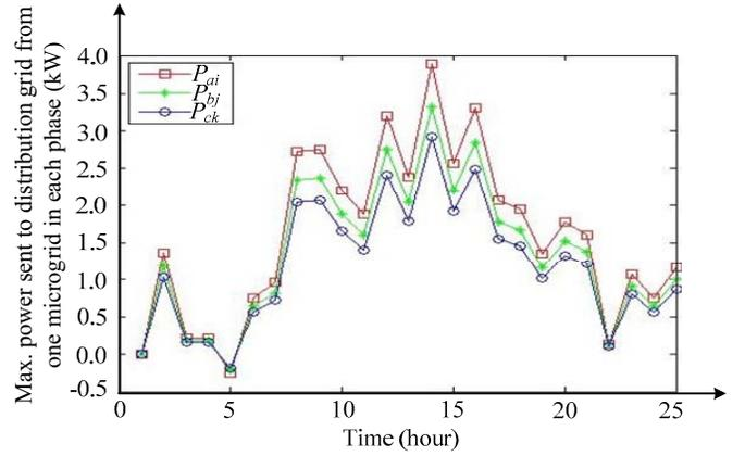
Fig. 5. The maximum power sent to the distribution grid by each microgrid in Phases A, B and C in each hour of a day.
