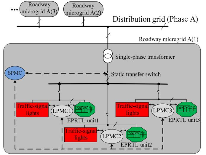
Fig. 1. Typical configuration of a single-phase roadway microgrid.
