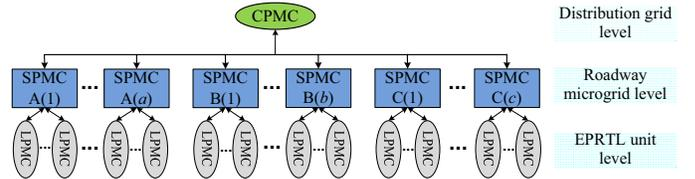
Fig. 3. Proposed hierarchical power management system.
