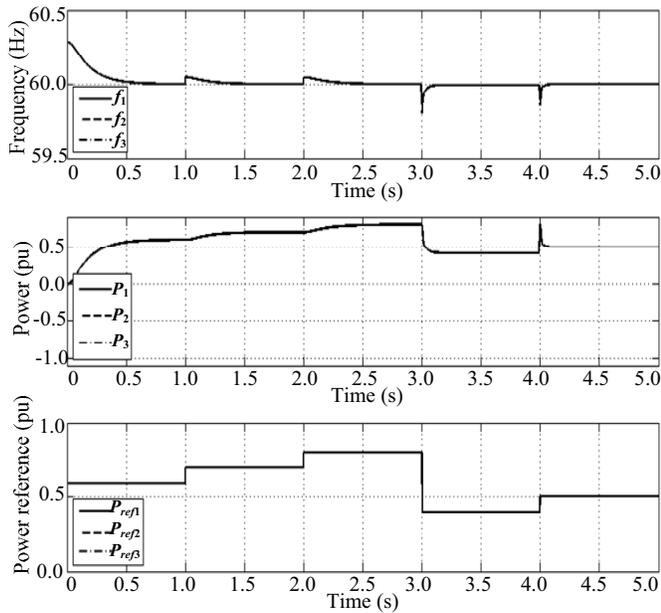
Fig. 7. Load changes from 1.2 pu to 1.5 pu and the reference power updates accordingly at 3 s and 4 s
