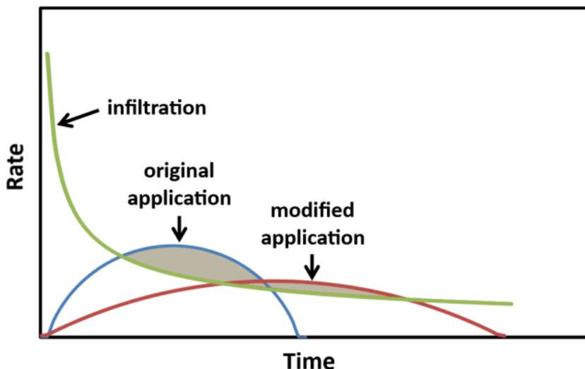
Figure 1. Runoff (grey area) caused by two different applications of the same irrigation depth
