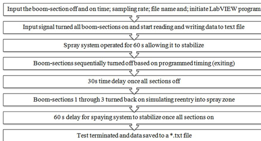
**Figure 2. Data collection procedure for the LabVIEW program.**
