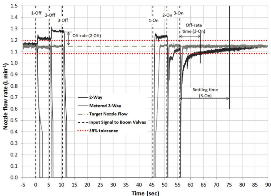
Figure 3. Nozzle flow response for the 2-way and metered 3-way boom valves when exiting and reentering  $70^\circ$  point rows at  $12.1 \text{ km h}^{-1}$  ground speed and  $112.1 \text{ L ha}^{-1}$  application rate.
