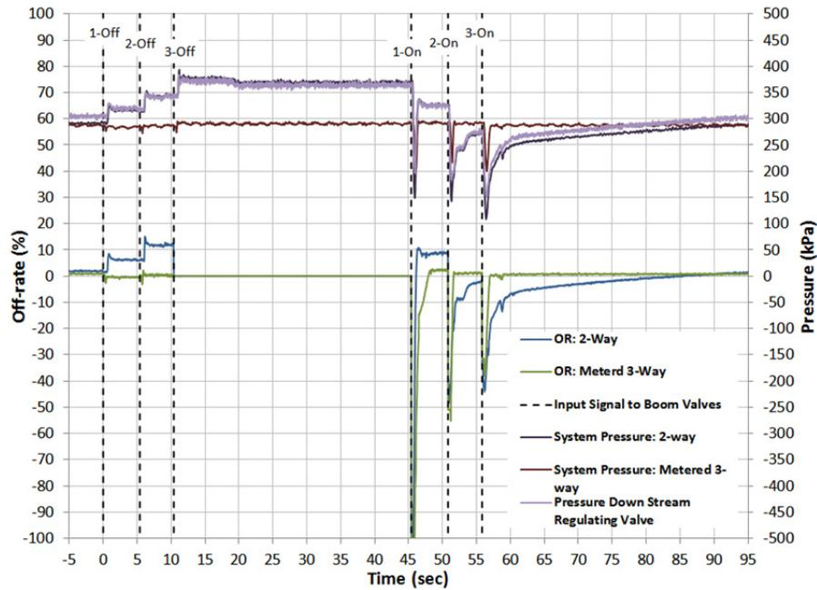
Figure 4. Pressure downstream of the regulating valve and nozzle off-rate for the 2-way and metered 3-way boom valve configurations when exiting and reentering 70° point rows at 12.1 km h<sup>-1</sup> ground speed and 112.1 L ha<sup>-1</sup> application rate.
