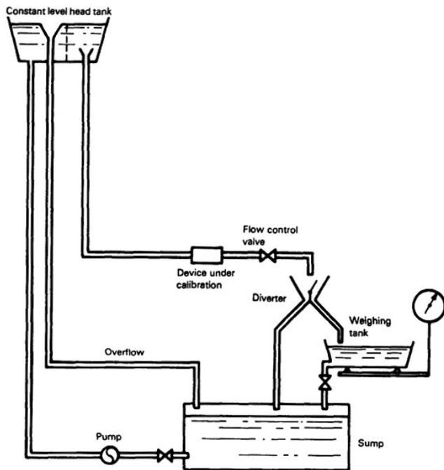
Figure 1. Schematic diagram of a static weighing system with constant head tank. Reprinted from MFC-9M-1988 (R 2006), by permission of The American Society of Mechanical Engineers. All rights reserved (ASME, 1988).
