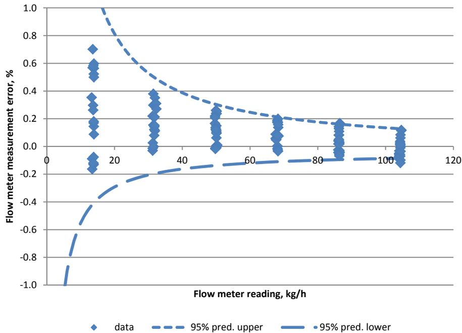
Figure 7. Flow meter errors and the 95% prediction band on a percent error basis for the static weighing calibration (with No. 2 diesel fuel) of the Coriolis Effect fuel flow meter used during PTO dynamometer tests of tractors at the Nebraska Tractor Test Lab.
