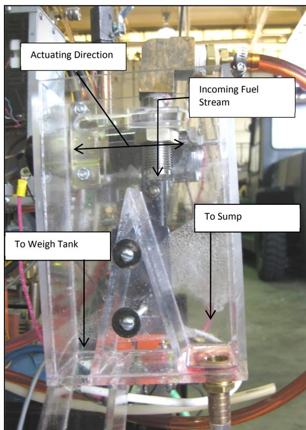
Figure 3. Flow diverter in the static weighing system of the flow meter calibration system at the Nebraska Tractor Test Lab.
