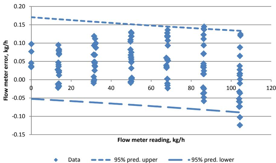
Figure 6. Flow meter errors and the 95% prediction band for the static weighing calibration (with No. 2 diesel fuel) of the Coriolis Effect fuel flow meter used during PTO dynamometer tests of tractors at the Nebraska Tractor Test Lab.
