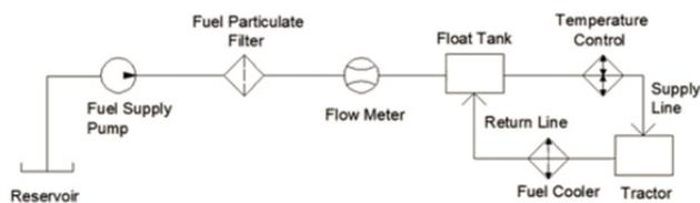
Figure 2. Schematic diagram of the fuel supply system during PTO dynamometer tests of tractors at the Nebraska Tractor Test Lab.
