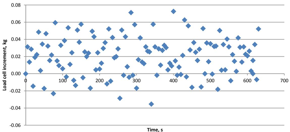
Figure 5. Load cell increments for the third replication of the 13.6 kg/h flow rate measurements using the dynamic weighing calibration method (with No. 2 diesel fuel) for the Coriolis Effect fuel flow meter used during PTO dynamometer tests at the Nebraska Tractor Test Lab.
