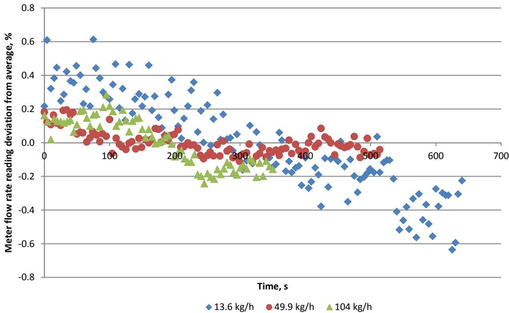
Figure 4. Meter flow rate reading deviations from average for the second replication of flow rate measurements using the dynamic weighing calibration method (with No. 2 diesel fuel) for the Coriolis Effect fuel flow meter used during PTO dynamometer tests of tractors at the Nebraska Tractor Test Lab.
