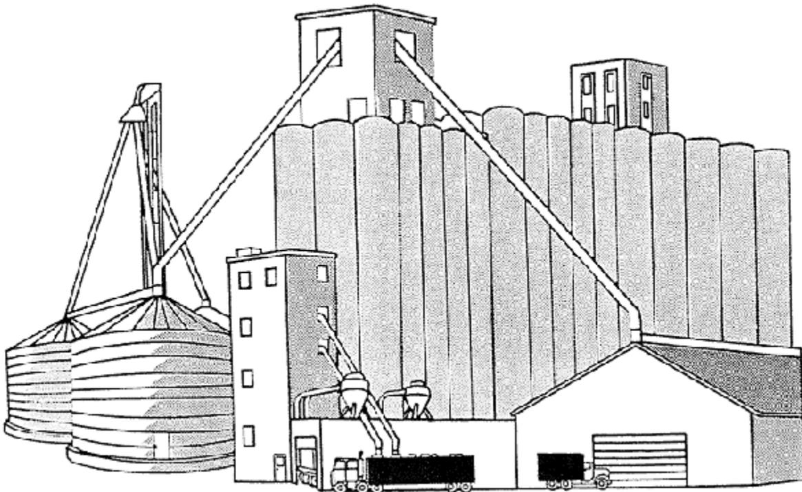
Any bucket elevator leg conveying grain is susceptible to grain dust explosions. The more grain conveyed with a particular leg, the greater the likelihood of a grain dust explosion. The possibility of a grain dust explosion exists in small on-farm legs, but it is much greater in larger commercial legs conveying millions of bushels of grain each year.
