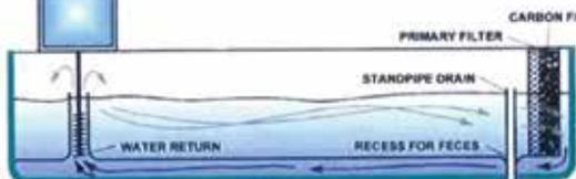
The Living Stream is a revolutionary design of recirculating water in a closed system. All the water in the insulated tank makes a complete cycle every 1-1/2 minutes, thus providing an equal amount of dissolved oxygen and the desired temperature throughout the entire tank.
