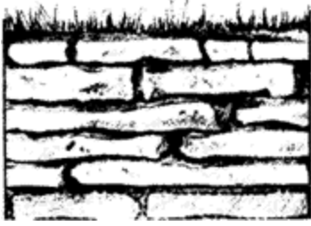
Properly constructed rock wall.
