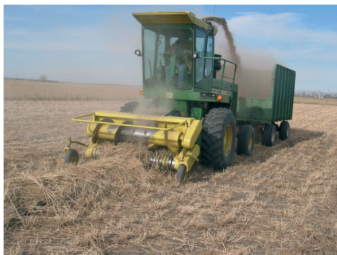
Figure 2. This field of Shawnee switchgrass was harvested to a 10-cm stubble height and chopped with a silage chopper equipped with a pick-up head in November.
