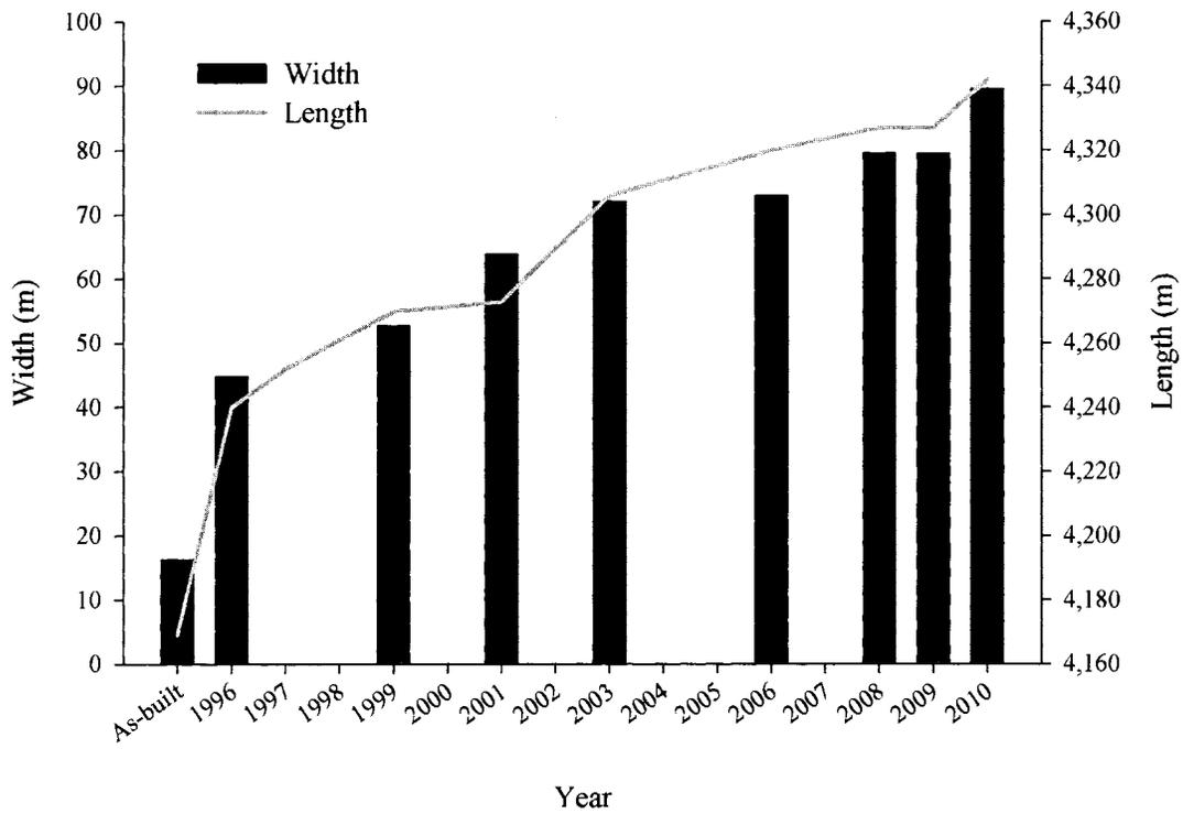
Figure 5. Width and length change at the Upper Hamburg Bend side channel from construction until 2010.
