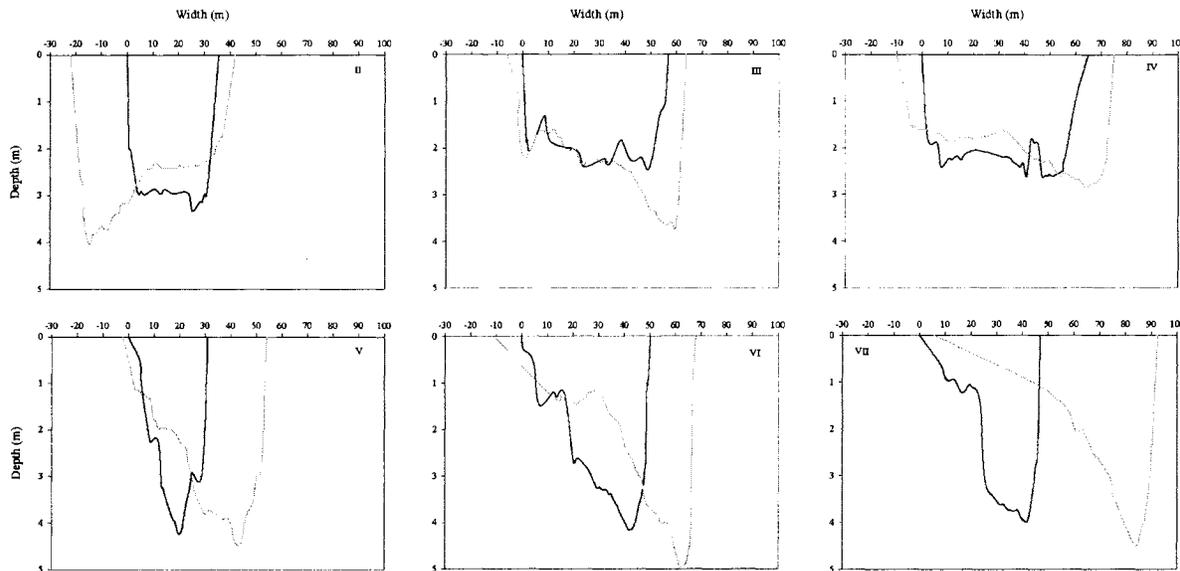
Figure 4. Longitudinal view of aggradation/degradation lines, Types II-VII, at the Upper Hamburg Bend side channel during the 2001 (black) and 2008 (gray) bathymetric surveys (2001 data from Jacobson et al. 2004). On all graphs, zero on the x-axis denotes the right-hand, descending bank during the 2001 survey. Negative numbers on the x-axis signify westward movement.
