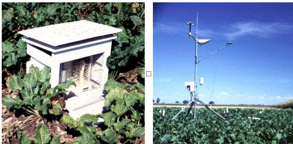
Figure 4. Weather instruments used for determination of DIV's in a sugar beet crop: (a) hygrothermograph and (b) automated weather station.
