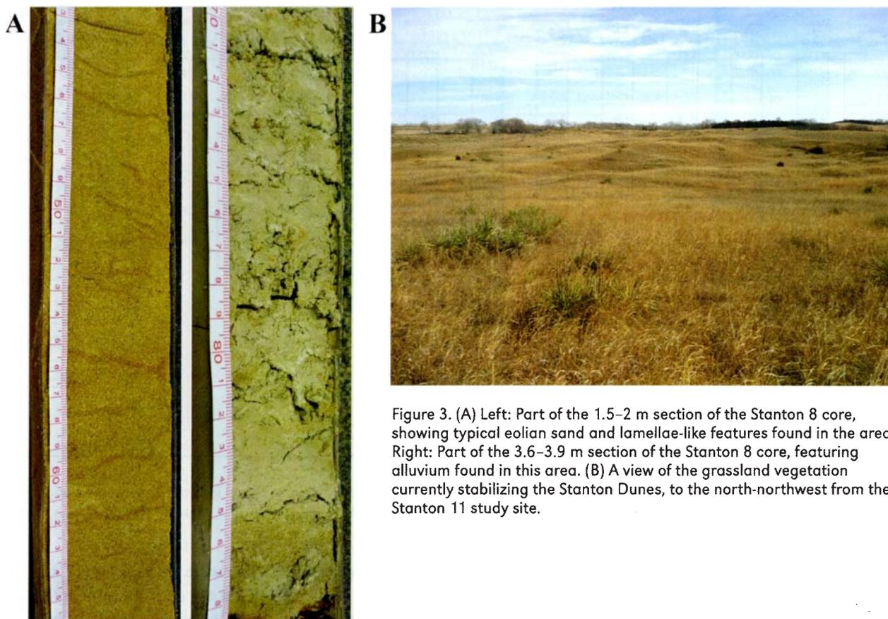
Figure 3. (A) Left: Part of the 1.5–2 m section of the Stanton 8 core, showing typical eolian sand and lamellae-like features found in the area. Right: Part of the 3.6–3.9 m section of the Stanton 8 core, featuring alluvium found in this area. (B) A view of the grassland vegetation currently stabilizing the Stanton Dunes, to the north-northwest from the Stanton 11 study site.
