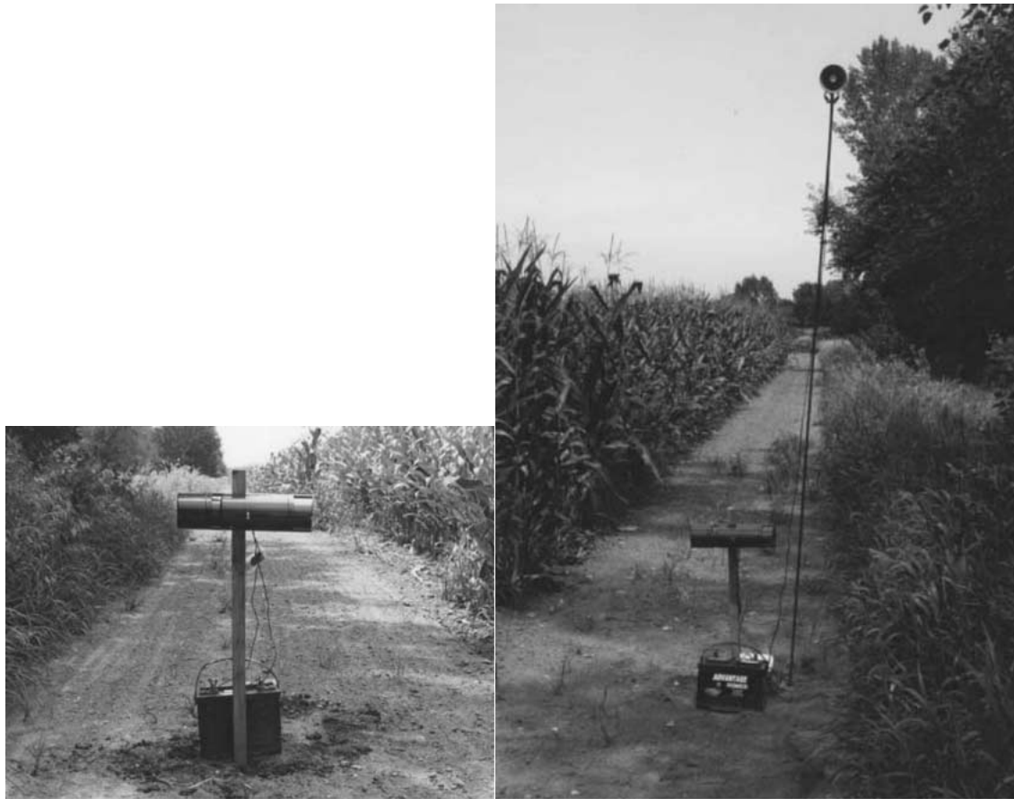
Figure 2. Infrared transmitting unit (left) and receiving unit (right) of the deer-activated bioacoustic frightening device that integrates an infrared detection system and a compact disk that repeatedly plays distress calls of white-tailed deer when activated.
